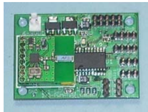
Figure 3: RRB with Sparkfun nRF module soldered
